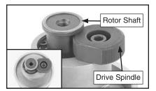
**Figure 12.** Sander in random orbital mode (pad removed for clarity).
